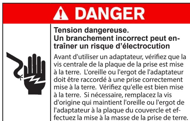
**L'UTILISATION D'UN ADAPTATEUR N'EST PAS AUTORISÉE AU CANADA. SI UNE PRISE DE MISE À LA TERRE N'EST PAS DISPONIBLE, N'UTILISEZ PAS L'APPAREIL JUSQU'À CE QU'UNE PRISE APPROPRIÉE SOIT INSTALLÉE PAR UN ÉLECTRICIEN QUALIFIÉ.**
