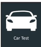
Use Car Test to perform Battery Tests on car batteries. Using test parameters the battery can be tested both in vehicle and out of vehicle. A System Test is also available for the in vehicle test. Press ▲◀▶▼ to return to the previous screen, select options and when necessary,  to enter or continue to the next step. Use **BACK** to return to the Main Menu.
