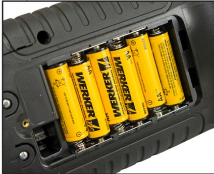
4. Remove the discharged batteries.
