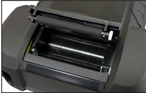
3. Place a new roll of paper in the compartment. The paper feeds from the bottom of the roll.
