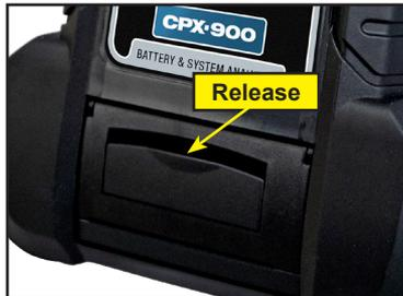
2. Lift the printer door and remove the spent roll.
